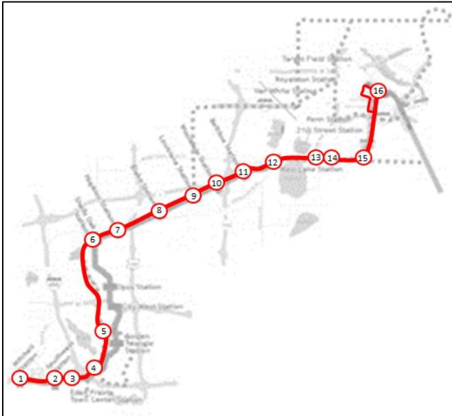
Southwest Main – Main route between Eden Prairie and Minneapolis – 5 Minute Service to Mpls 15.5 hrs/day, from Mpls 12 hrs/day – 2.487 million miles/yr, 31.5%; 100,100 hrs/yr, 20.4%.
